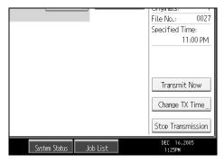
Press [Clear], re-enter the transmission time using the number keys, and then press [OK].
